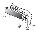
Press the left side © of the DCP carefully to fit it in place.
